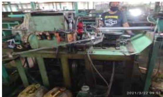
**Gambar 5.** Mesin *spiral finned tube*
